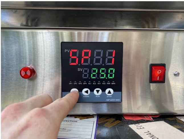
This will show SP1 above and the starting temperature of the program at the bottom. In order to change this value you need to use the 3 arrow keys. The down (run) key will decrease the selected digit, the up (stop) key will increase the selected digits.
