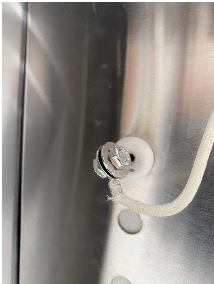
Detail of a single terminal: the element tail is formed into a closed loop pre-loaded against the ceramic insulator. A stainless bolt passes through the loop to make the connection. Tighten firmly but do not overtighten, and keep the cut-off tail clear of the casing and cover.
