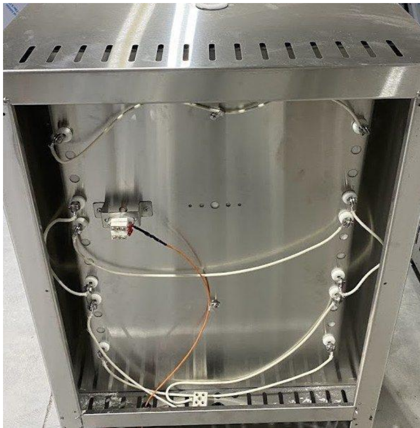
Element terminations at the rear of the case: element tails pass through ceramic feed-throughs and are secured at the terminal posts. Note the routing of the connecting wires and the thermocouple block in the centre.
